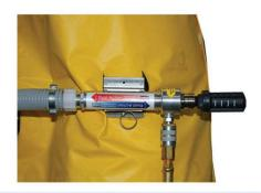
Heating Mode Configuration. Muffler is placed on the cold end of the unit.
